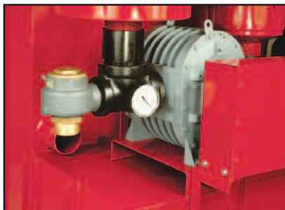
Powerful positive displacement blower.
